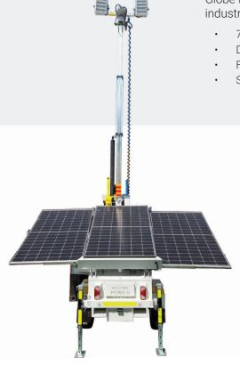
Globe Power's Eco GP56K Hybrid Solar Lighting Tower has been built to suit various industries. With a Hatz backup engine it can run in any weather.
